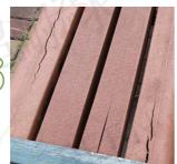
Absorb water Deformation fracture
